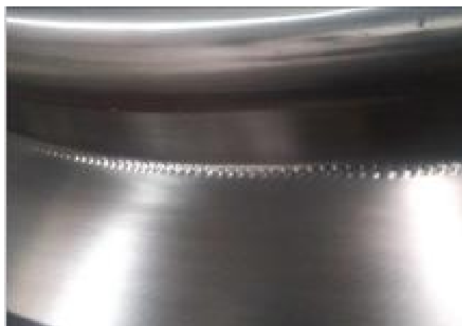
Argon shielded welding line
